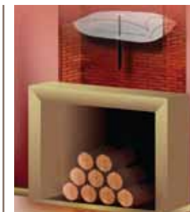
Above: Diagram showing an expanded chimney balloon inserted into the flue. Unlike a draught excluder sheet or 'blanket', a chimney balloon is concealed out of sight.
