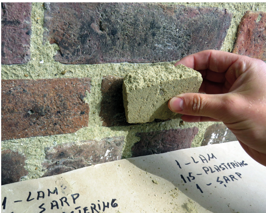
Approved lime mortar 'biscuit' sample
